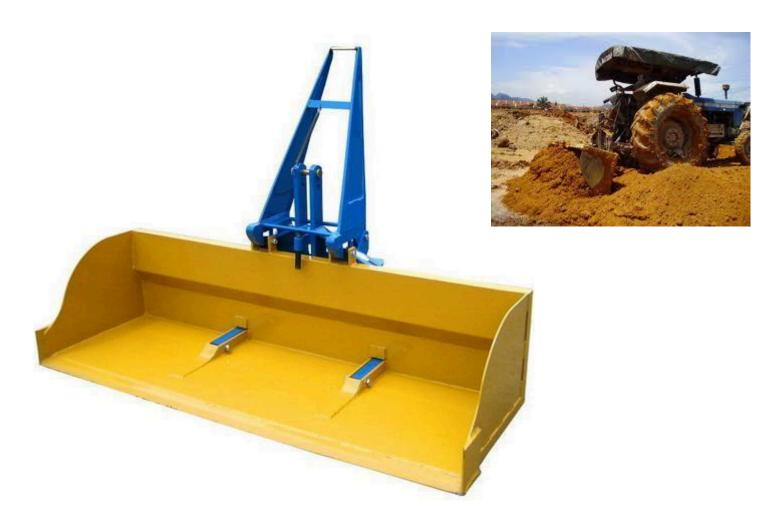
The ANSONFARM Tractor 3 point linkage mounted rear bucket is suitable for tractors. Models are available in various sizes. Working in reverse, the bucket may be tipped to unload earth. The machine is constructed of steel, a grader blade cutting edge is welded. Ideal for leveling land, Cleaning harvester's paths, moving earth, building bunds both in plantations or construction sites.
